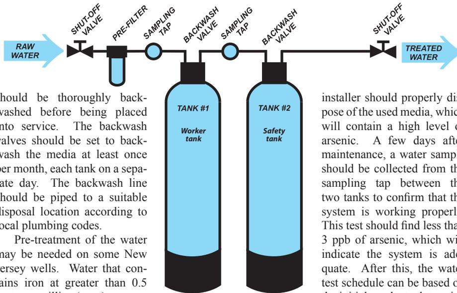
should be thoroughly backwashed before being placed into service. The backwash valves should be set to backwash the media at least once per month, each tank on a separate day. The backwash line should be piped to a suitable disposal location according to local plumbing codes.
